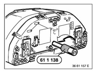
Remove complete instrument carrier, refer to 62 21 000.
